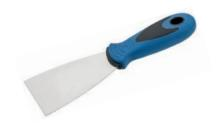
Info: Flexible stainless steel blade. Comfortable plastic handle. Elastic properties of the blade are due to the flexibility of metal. The metal is thickerat the handle base and thinner at the end of the blade.
